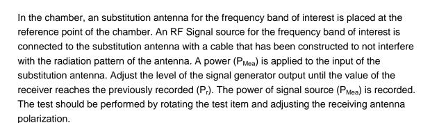
4. The Path loss (P<sub>pl</sub>) between the Signal Source with the Substitution Antenna and the Substitution Antenna Gain (G<sub>a</sub>) should be recorded after test.
