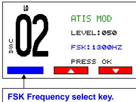
Step-2. Select the FSK Frequency [1300Hz] by **FSK Frequency select key**.
