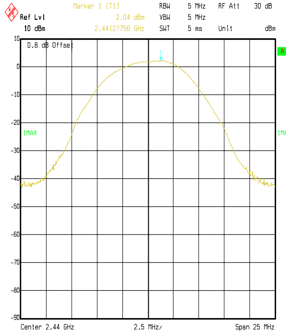
Title: Raymarine EUT: Smart Controller. Peak Power FCC P15.247 Comment A: 46813 Middle Channel Date: 24.NOV.2004 13:54:28
