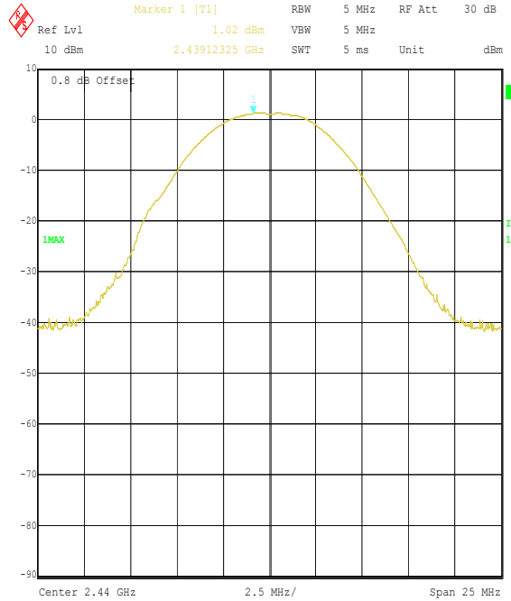
Title: Raymarine 46813JD10 EUT S1000 Autopilot FCC P15.247 Comment A: Peak Output Power Middle Channel Date: 4.JAN.2005 13:59:23
