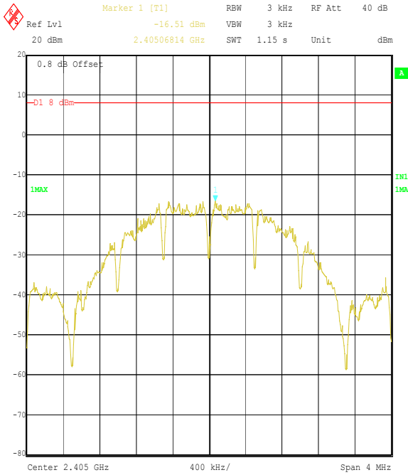
Title: Raymarine 46813JD10 EUT S1000 Autopilot FCC P15.247 Comment A: Peak Power Spectral Density Bottom Channel Date: 4.JAN.2005 13:55:47
