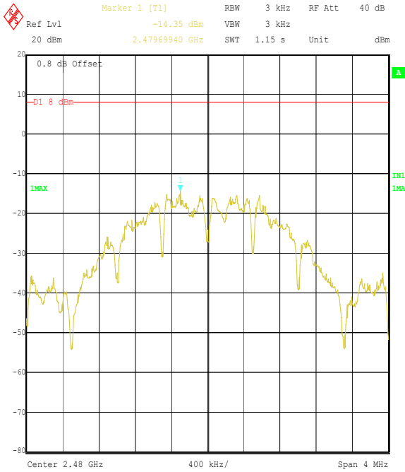
Title: Raymarine 46813JD10 EUT S1000 Autopilot FCC P15.247 Comment A: Peak Power Spectral Density Top Channel Date: 4.JAN.2005 13:54:34
