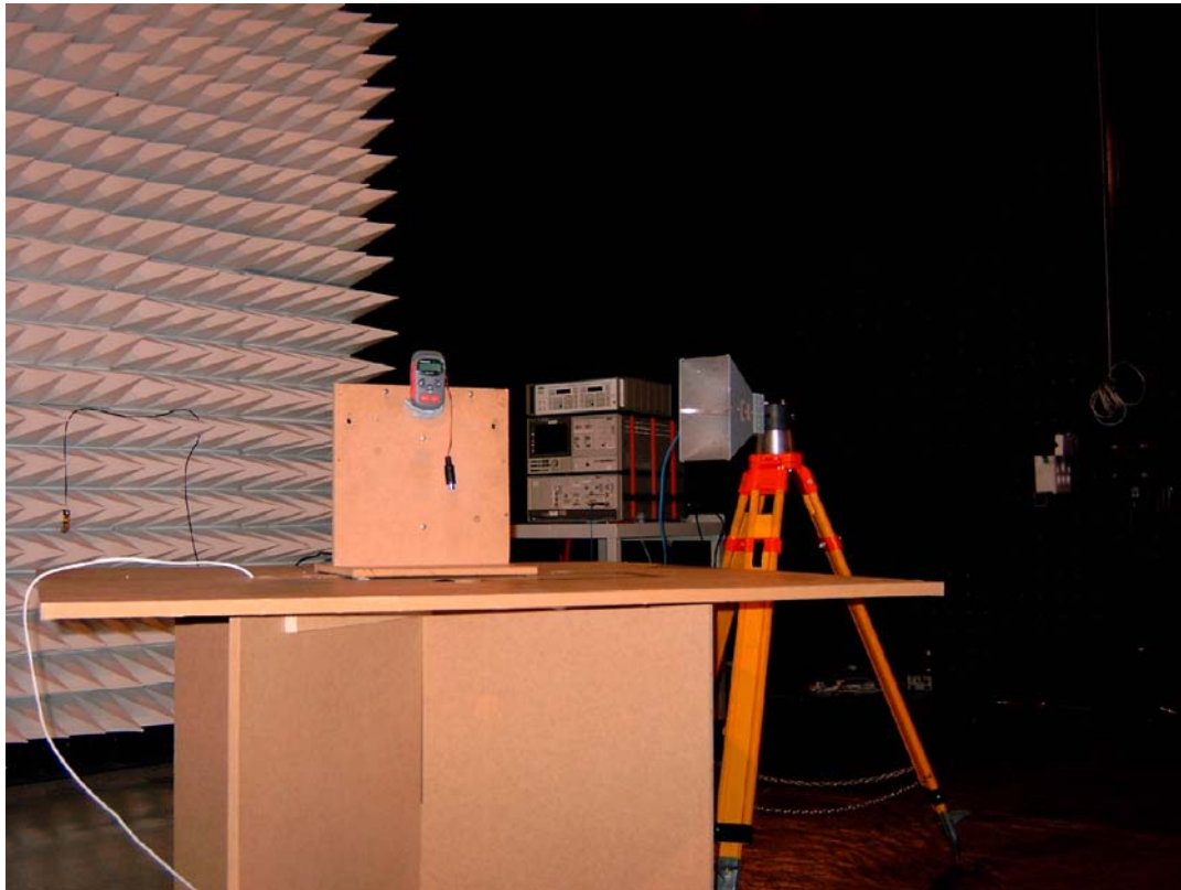
Figure 4 Set up showing measurements above 7GHz at 1m.
