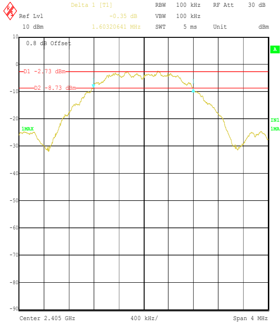
Title: Raymarine 46813JD10 EUT S100 Controller FCC P15.247 Comment A: 6 dB Bandwidth Bottom Channel Date: 4.JAN.2005 14:16:31
