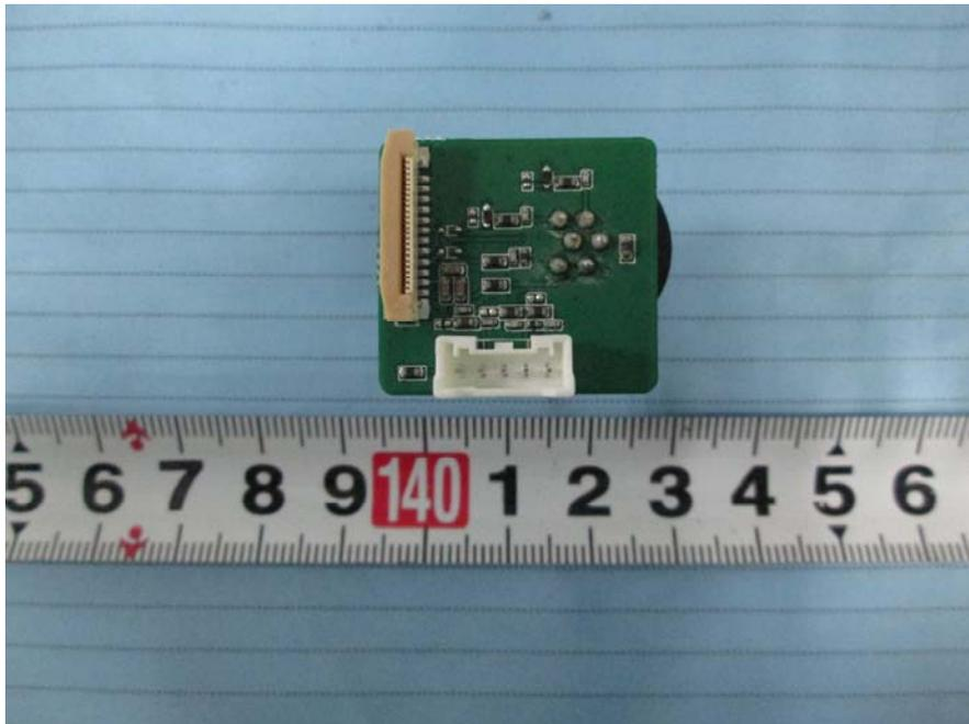
**EUT –Microphone Cover off View**
