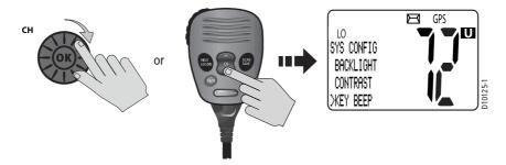
5. Press **CH/OK** on the transceiver or the **HI/LO** key on microphone to accept. The options under that sub-menu are displayed.
