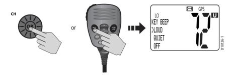
6. Rotate the **CH/OK** knob on the transceiver or press the **CH** up/down key on the microphone to highlight the desired option.
