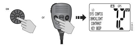
4. Rotate the **CH/OK** knob on the transceiver or press the **CH** up/down key on the microphone to highlight the desired sub-menu.
