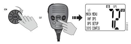
3. Press in the **CH/OK** knob on the transceiver or **HI/LO** key on the microphone to accept. The sub-menu headings are displayed.
