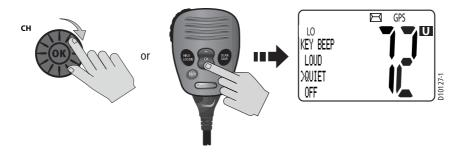
7. Press **CH/OK** on the transceiver or the **HI/LO** key on the microphone to accept. The setting is changed. Continue in the same manner to make any other setting changes.
