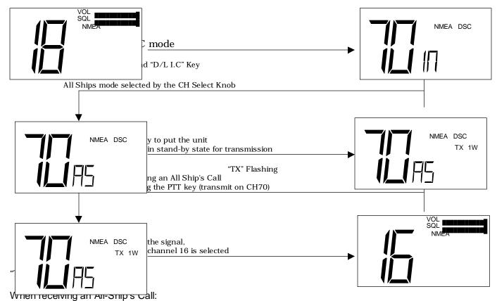
a) A tone will sound and the radio will enter the DSC mode with "as" flashing. Press the DSC key once and the radio will automatically select channel 16. There is no acknowledge required for an All-Ship's Call.
