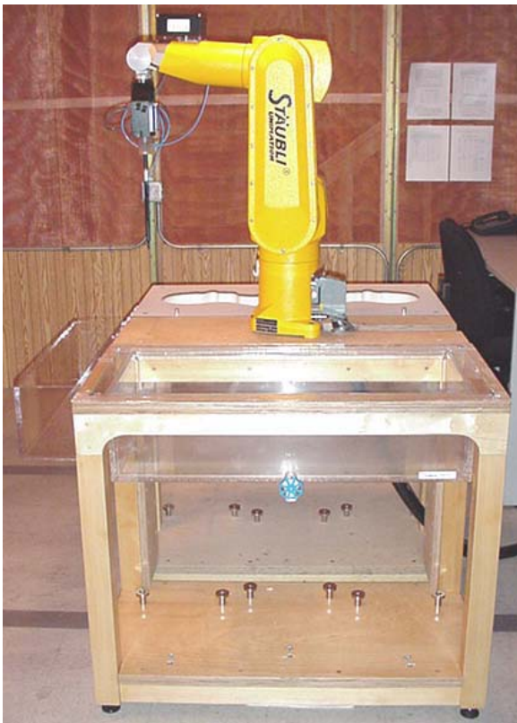
DASY4 SAR Measurement System with validation phantom
