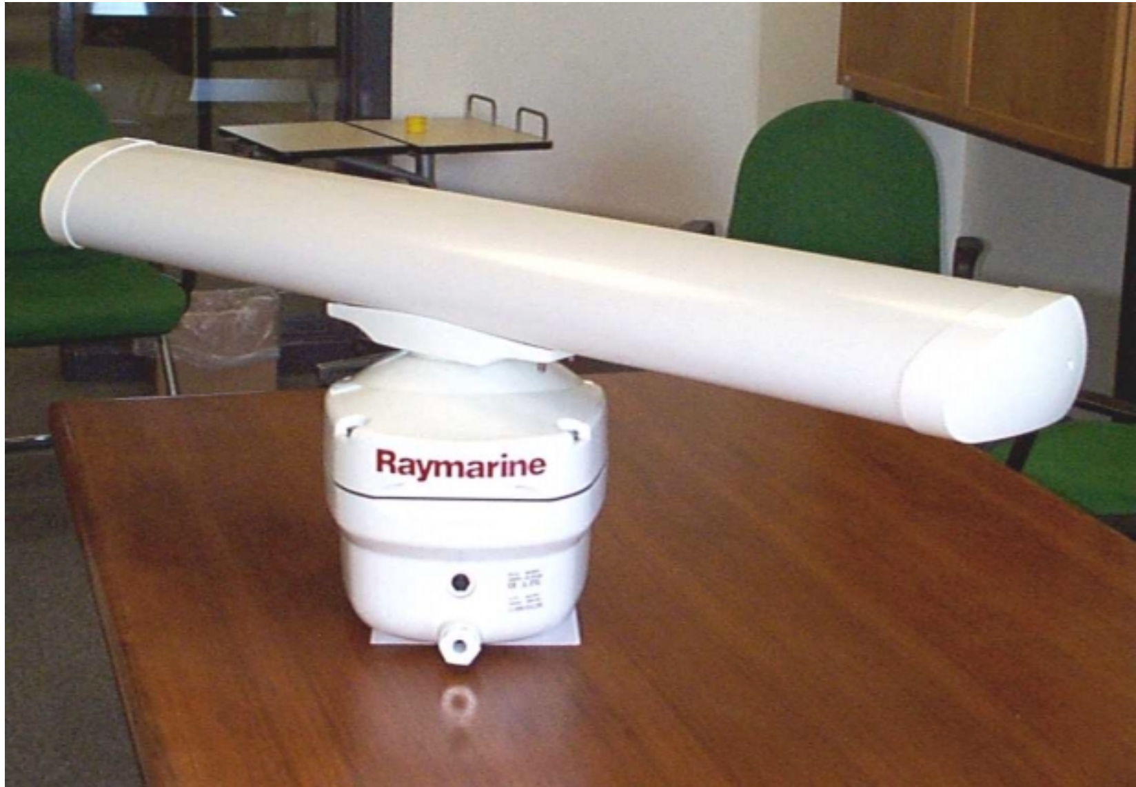
10kW, 48" Open Array Scanner Unit
