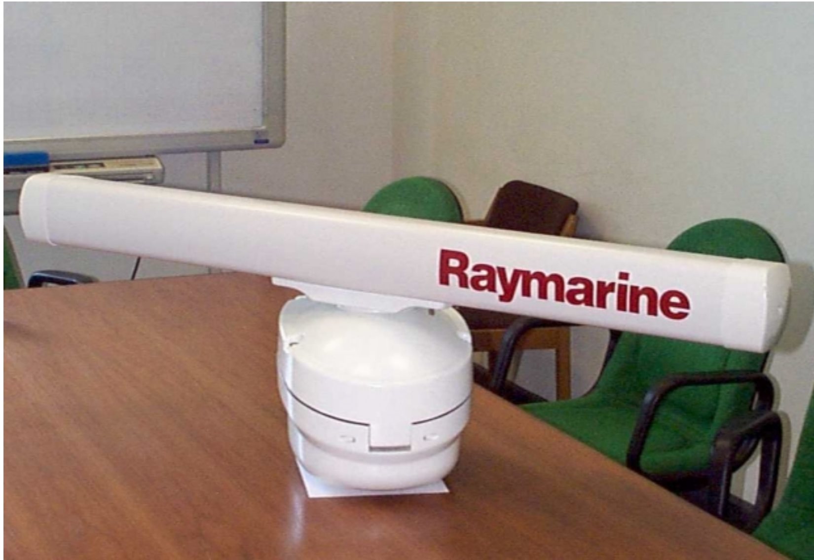
10kW, 48" Open Array Scanner Unit
