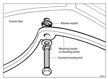
You may need to use longer M8 mounting bolts to secure the scanner if you have used shims to lower the radar beam.
