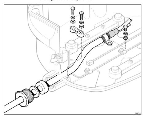
6. The cable is supplied prepared and ready to fit to the signal and power connectors. If you need to cut the cable to length, strip off the protective outer sleeve then use the supplied kit to prepare the cable as detailed in the following illustration.
