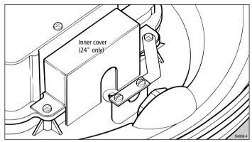
Remove the drain tube from inside the base of the scanner, and insert it into the drain hole as shown in the following diagram.
