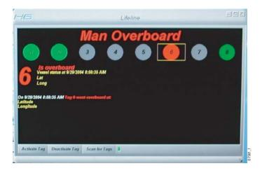
In the event of an alarm, the Lifeline data box will automatically expand onto the left hand screen. It will show which tag has alarmed and give details of time position, and the boat's speed at the time of the alarm. A Man Overboard marker will also be placed on the chart screen.
