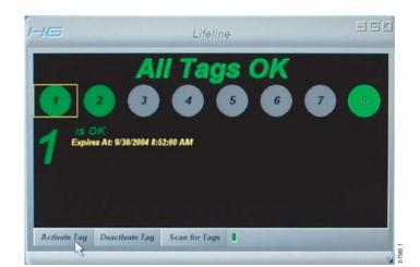
Activated tags are shown in green, inactive tags are shown in grey. Moving the cursor over a tag indicator will cause a yellow box to appear around it. Information for that tag is then displayed in the databox.
