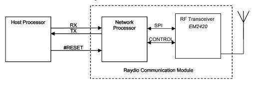
The Raydio Communication Module (RCM) is based upon Ember's EM2420 2.45GHz RF transceiver connected to an ATMEGA64 microprocessor, the Network Processor. This Network Processor runs EmberStack - Ember's networking embedded wireless networking solution.
