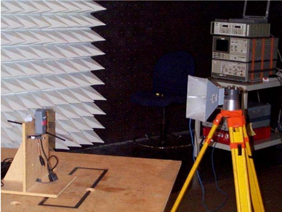
Figure 6 Set up showing measurements above 7GHz at 1m.
