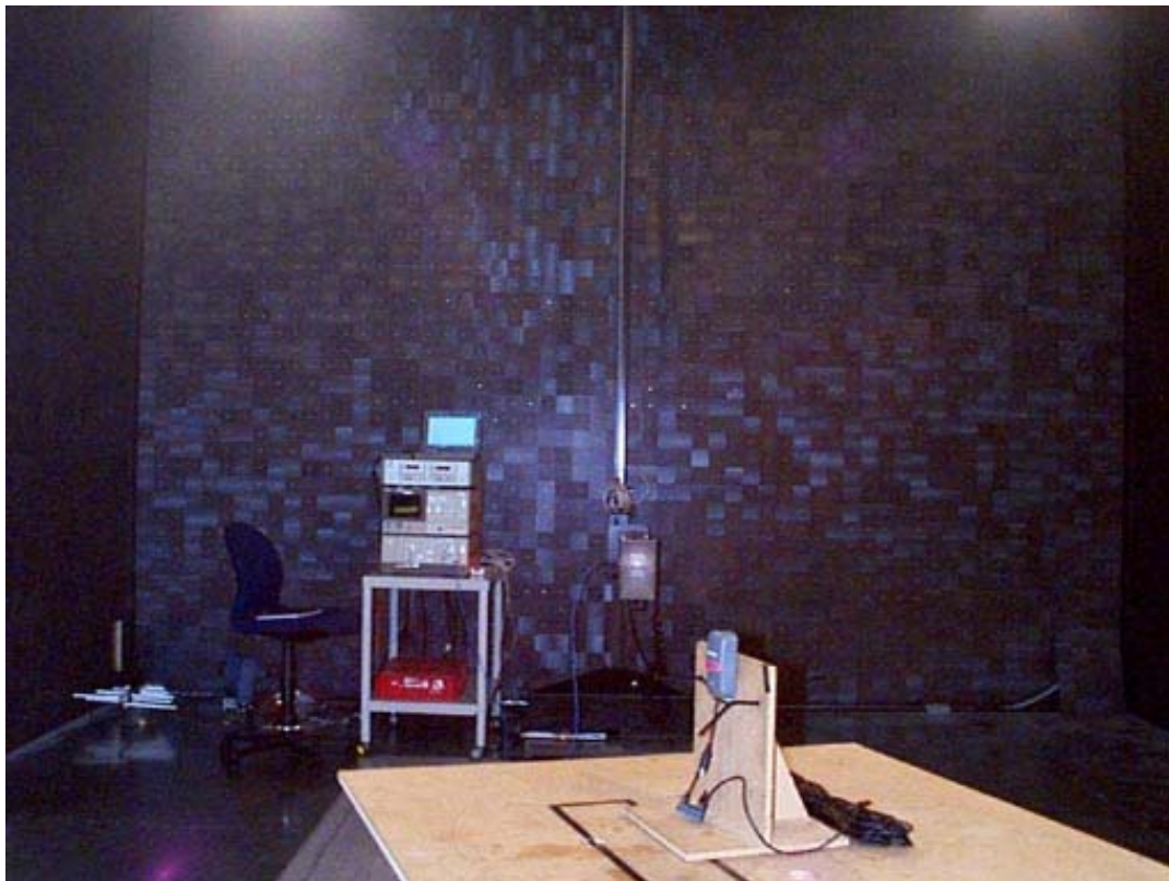
Figure 5 Set up in chamber for 2GHz-7GHz measurements at 3m.
