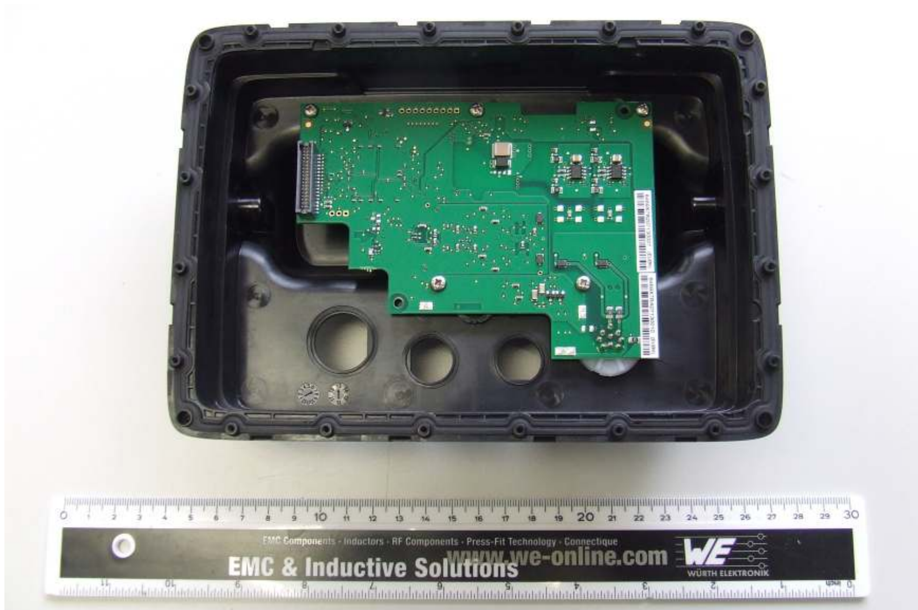
Figure 7 - Inside of A7 rear casing showing Sonar PCB
