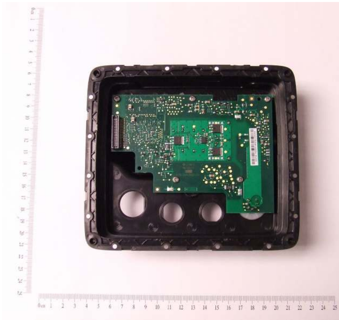
Figure 6 - Inside of A6 rear casing showing Sonar PCB
