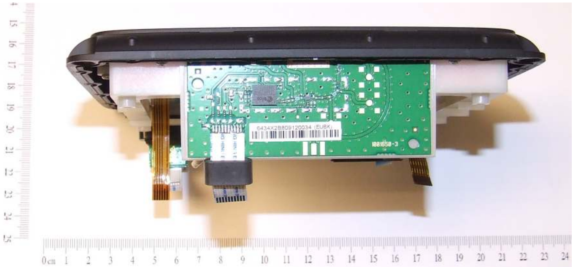
Figure 23 - GPS PCB (fitted)
