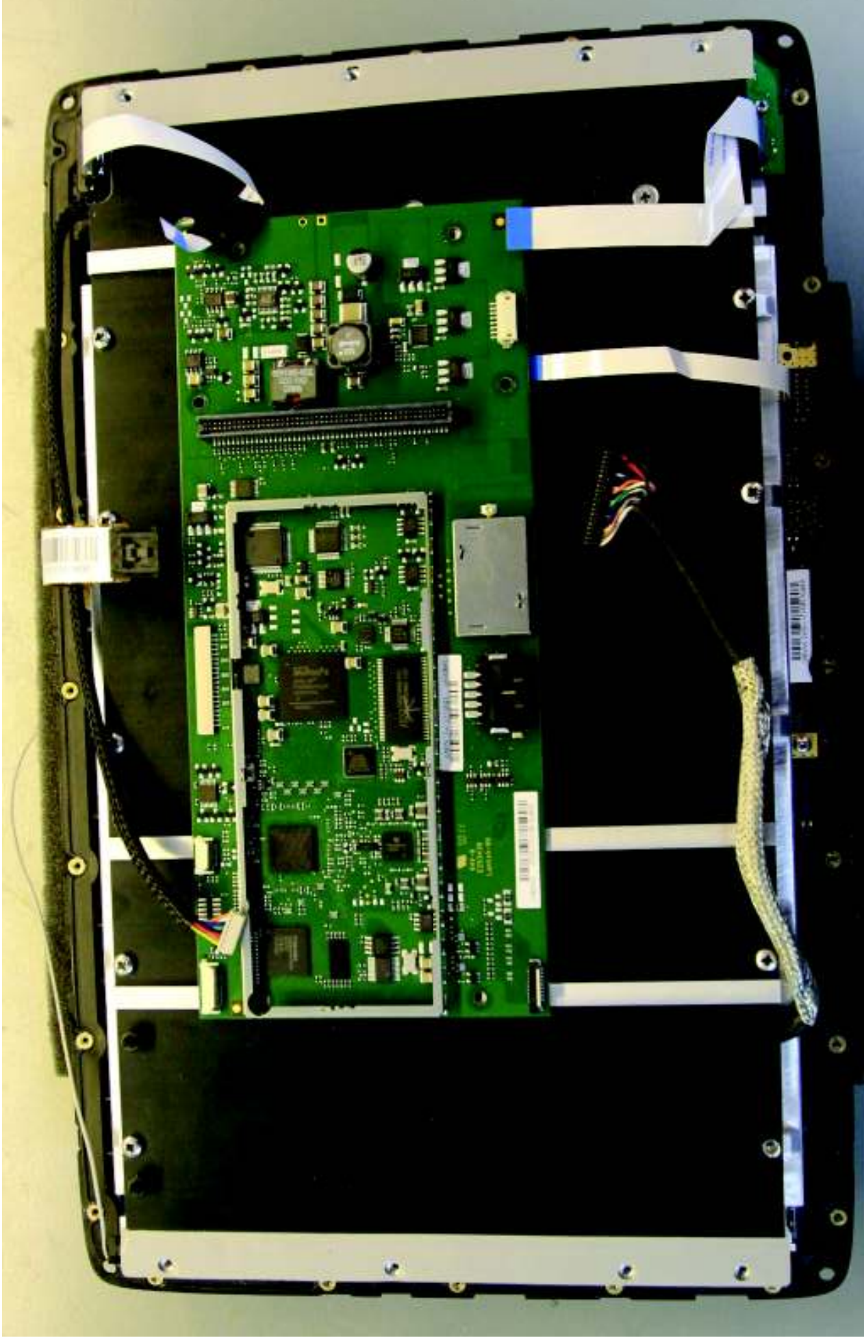
Figure 9 - Rear of 12 inch LCD with heatsink and location of CPU board.
