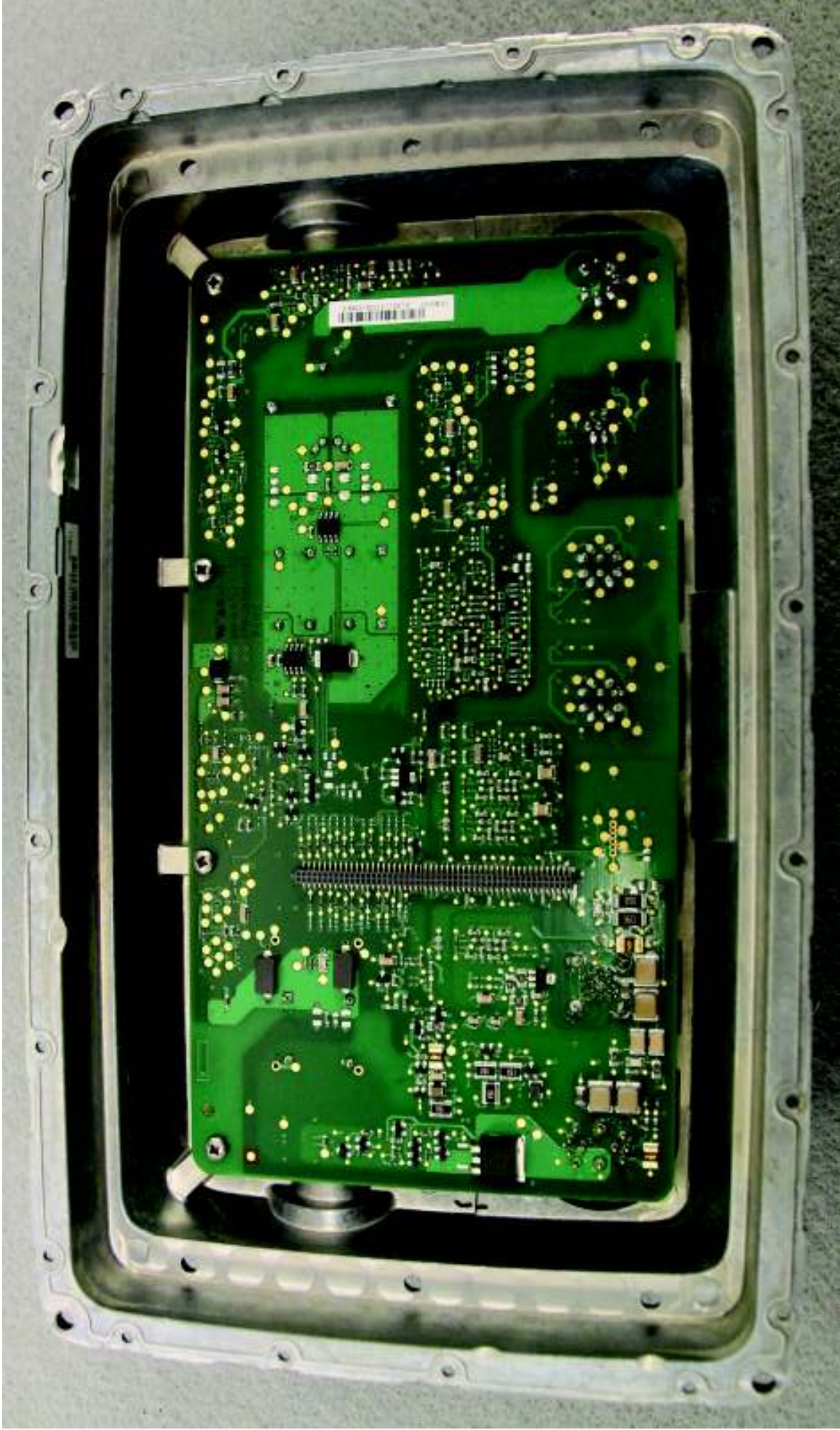
Figure 25 - inside of rear casting with connector / sonar board fitted
