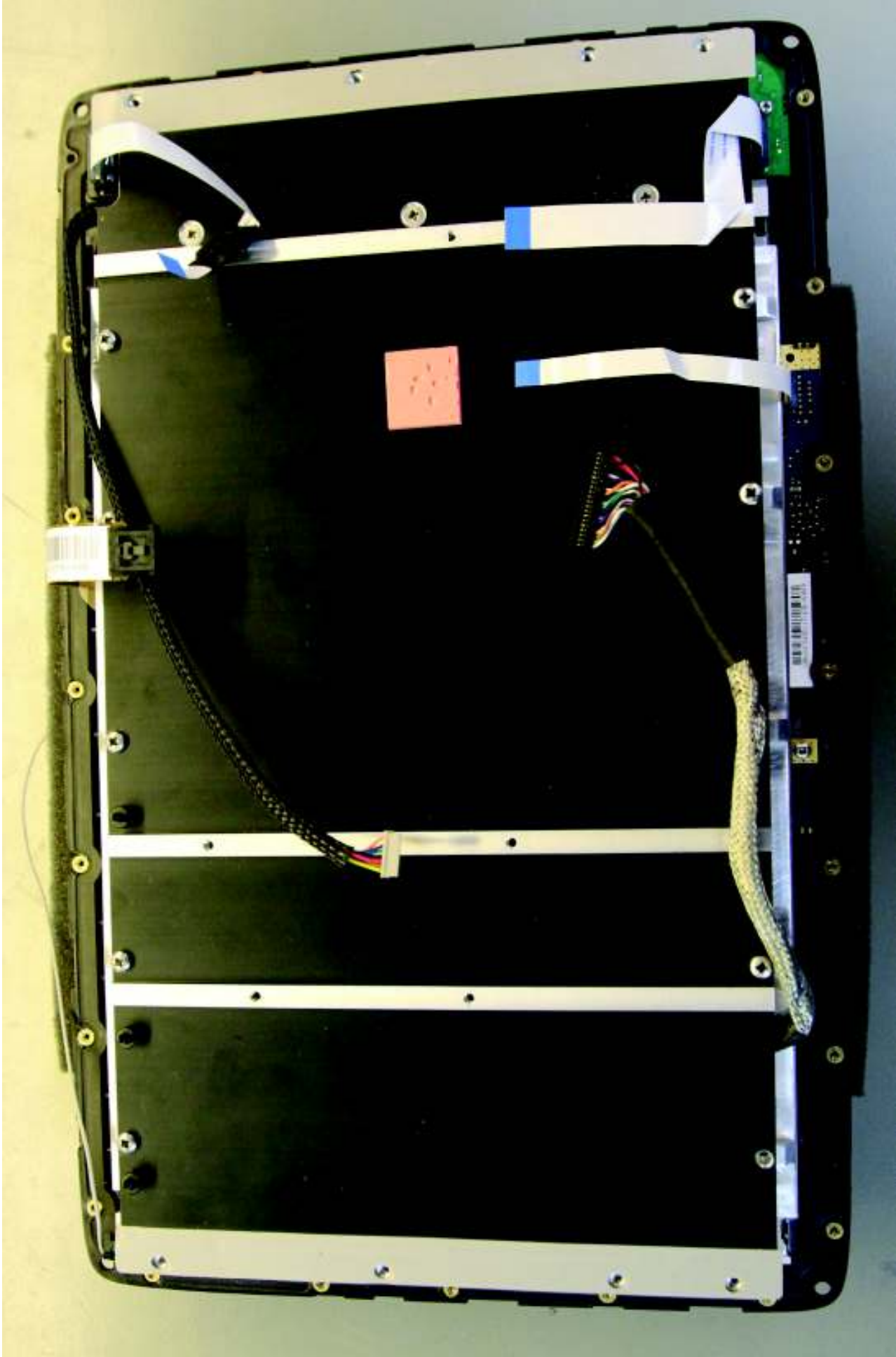
Figure 8 - Rear of 12 inch LCD with heatsink fitted
