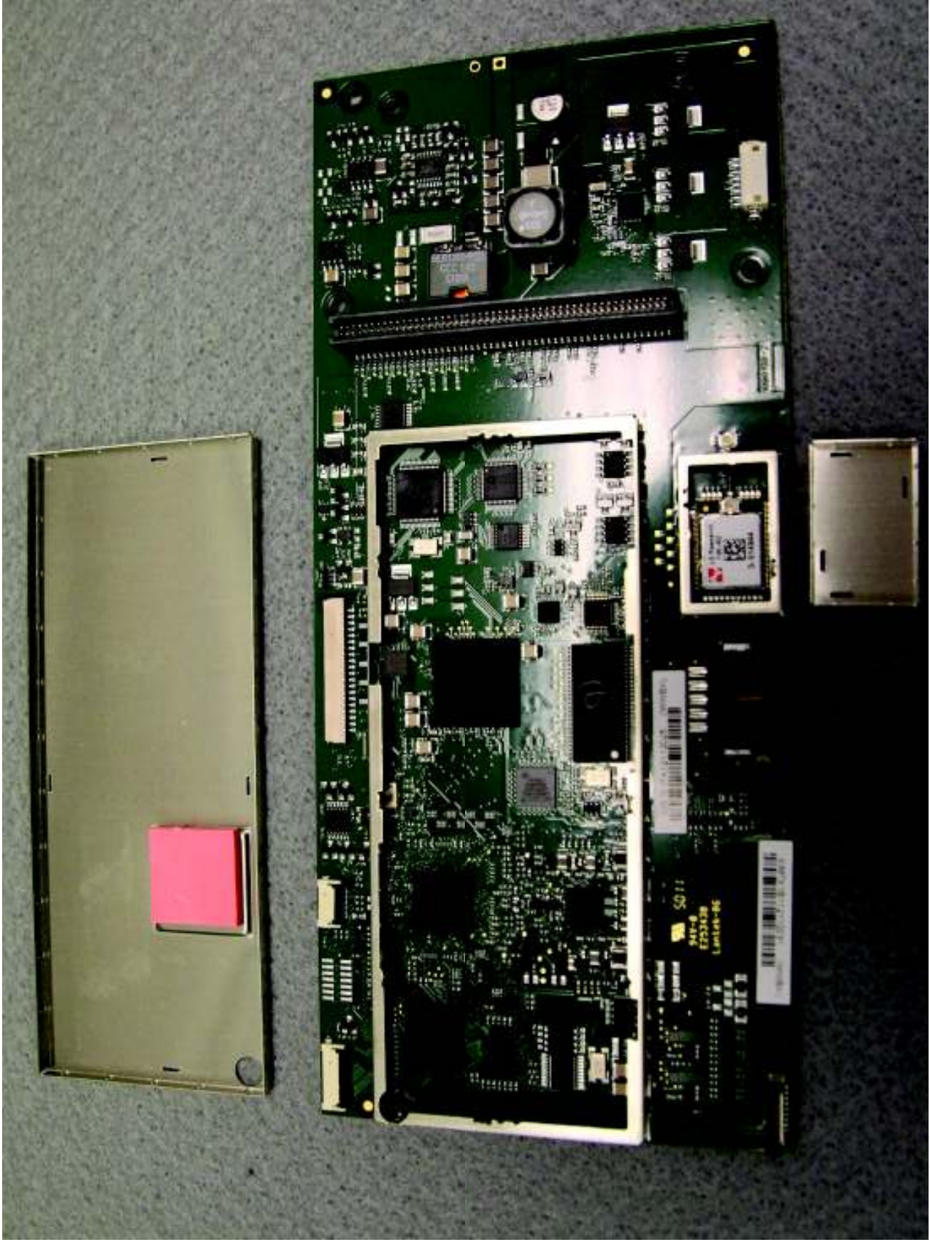
Figure 12 - Top of CPU PCB - cans removed
