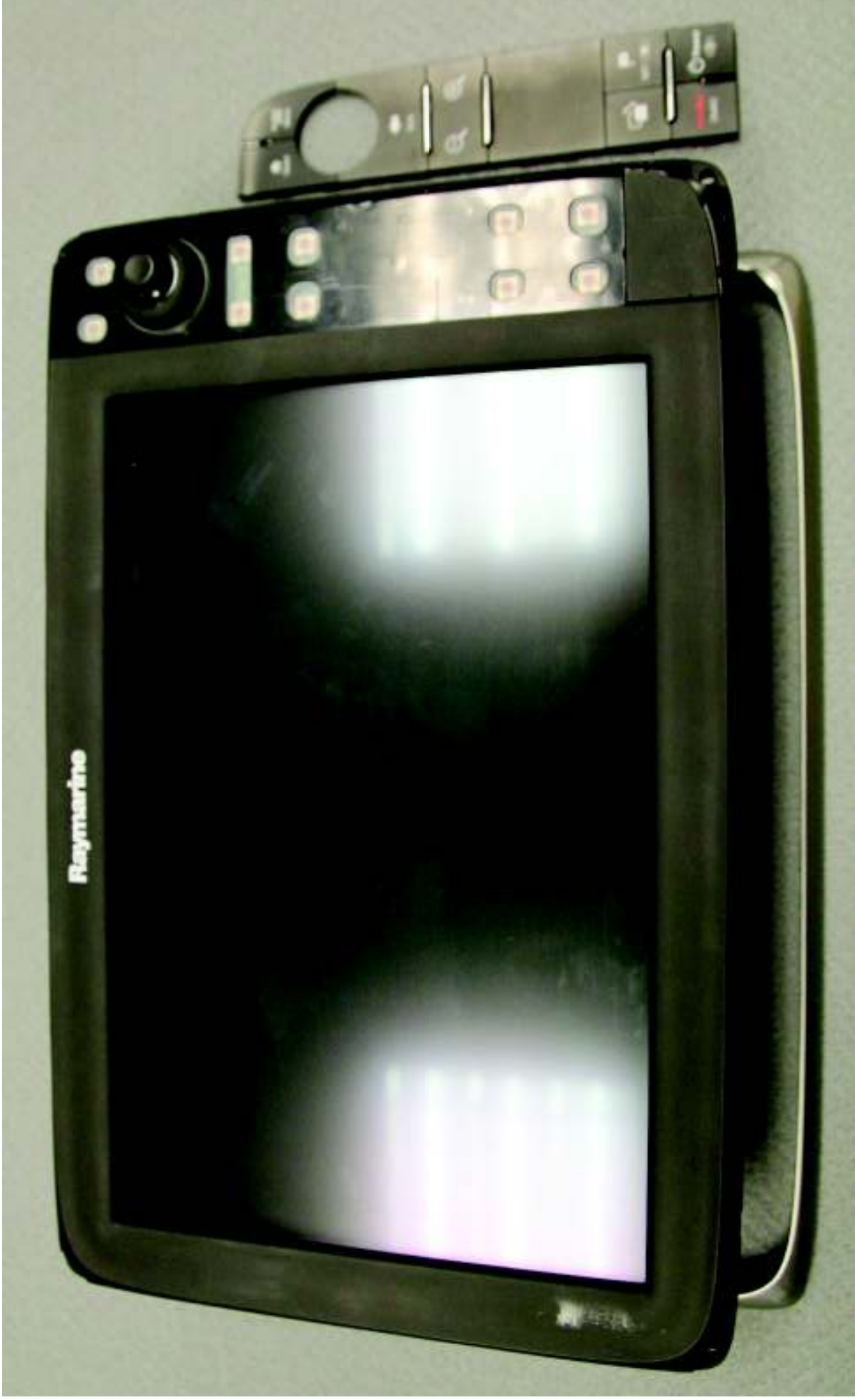
Figure 1 - 12 Inch unit - keypad and fascia removed
