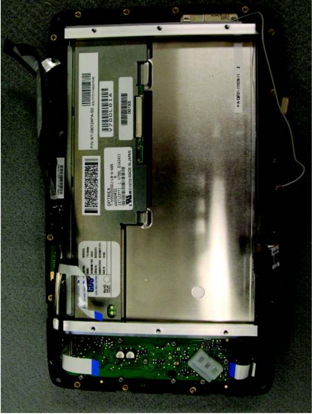
Figure 27 - 9 inch LCD rear with heatsink removed
