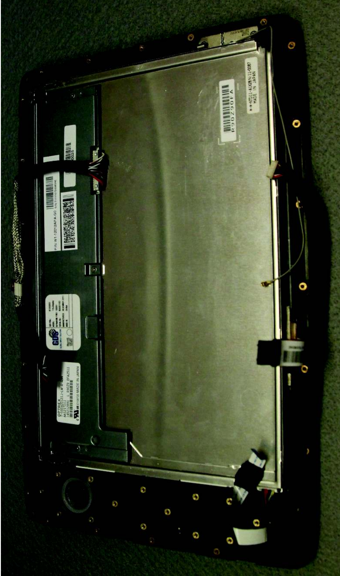
Figure 7 - read of 12 inch LCD - heatsink removed
