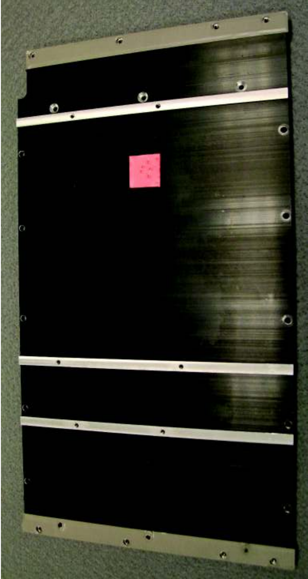
Figure 14 - 12 inch internal heatsink – top
