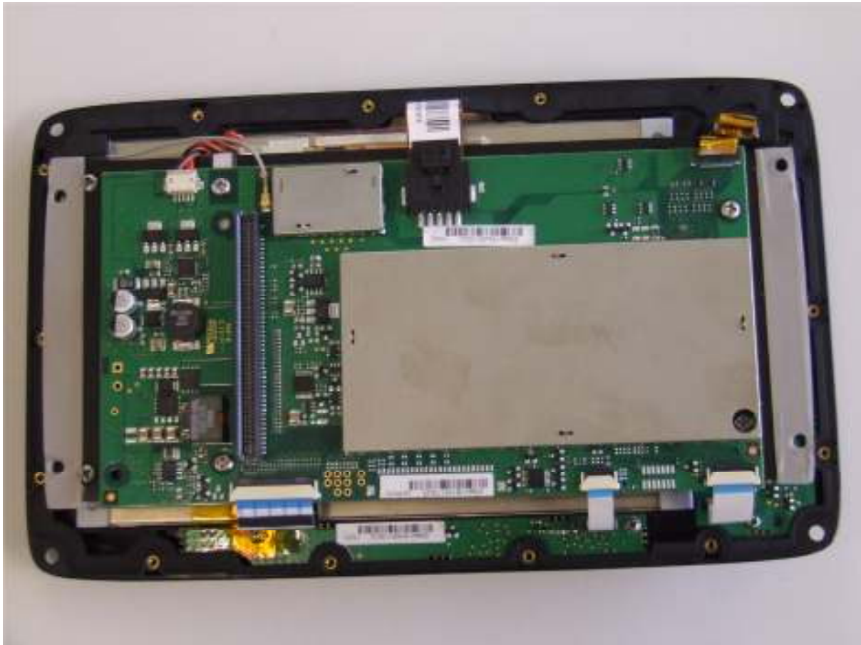
Front half of unit, CPU PCB fitted to heatsink on rear of LCD module
