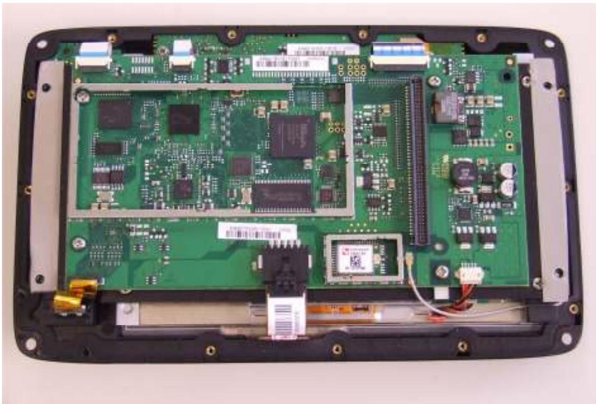
Processor board with cans removed
