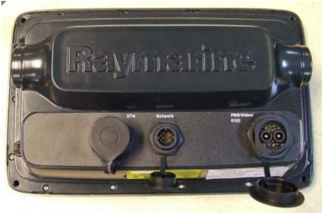
Rear of Chartplotter display with facia removed
