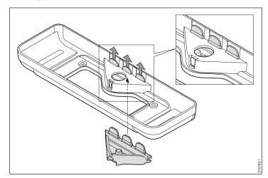
3. Fit the battery, taking care to avoid contamination of the cover seal.
