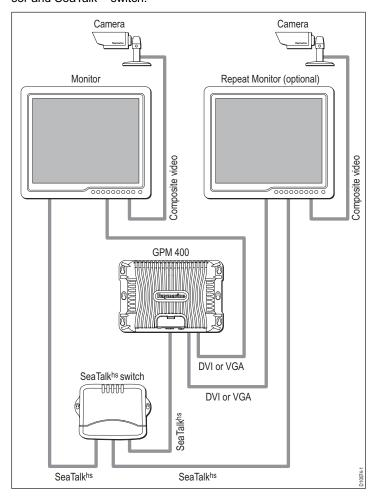
Monitors may be connected to the GPM400 using either VGA or DVI cable.
