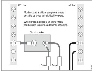
The fuse must be of an appropriate type and rating for the load to be protected.
