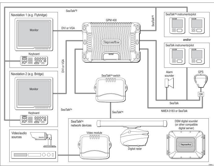
**Note:** Where 2 displays are connected to a single processor, both will display the same information.
