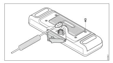
5. For charging and wired operation use the cable provided **Note:** The keyboard should be charged for 6 hours before use.
