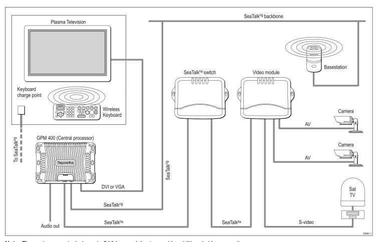
Note: The system may include up to 2 Video modules to provide additional video capacity.
