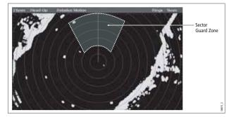
You can adjust the sensitivity of guard zones on the Alarms Setup Menu. For more information, see *Alarm Setup Menu* on *page 194*.
