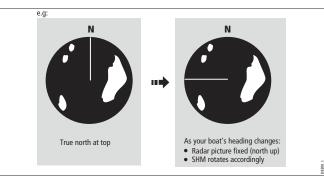
If heading data becomes unavailable while in this mode, a warning message will be shown, the status bar shows North-Up in brackets and the radar uses 0° heading in relative motion. When heading data becomes available once more, North-Up mode is reinstated.
