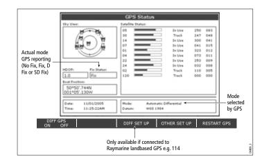
GPS accuracy depends upon the parameters shown, especially the azimuth and elevation angles which are used in triangulation to calculate your position.
