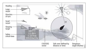
Vectors can be displayed for each target. These vectors indicate the direction of travel and rate of turn of the vessel and the distance it will travel over a specified period of time (COG/SOG vector). Targets displayed with their vectors are referred to as 'active targets' and are scaled according to the size of the vessel.
