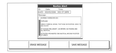
When you receive a message, the toolbar gives you the option to erase or save the message as appropriate. The G-Series system can save up to 100 Navtex messages. Once this capacity is reached, it starts to overwrite the oldest messages with newer ones.
