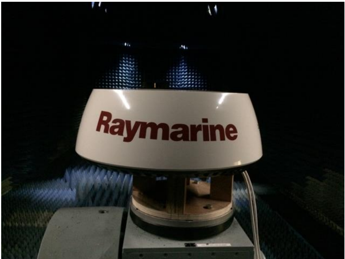
Figure 2-1 – Radar system during test within the anechoic chamber at QinetiQ Funtington
