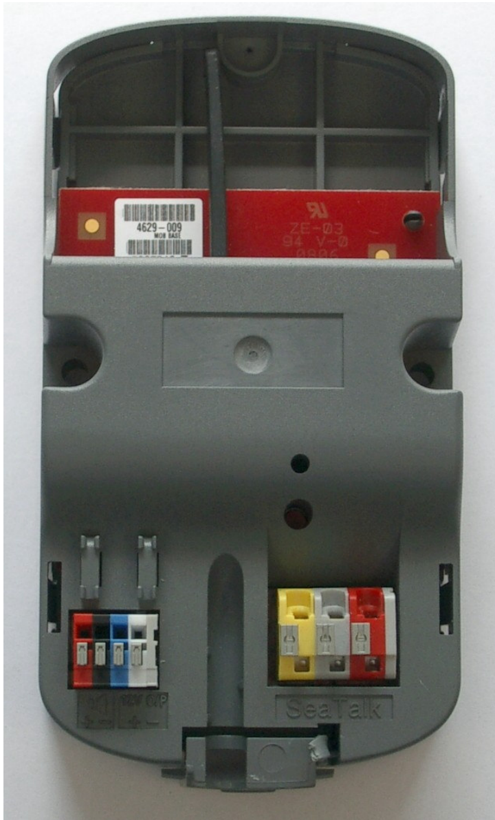
LT Base Station Front View, Primary Cover Removed
