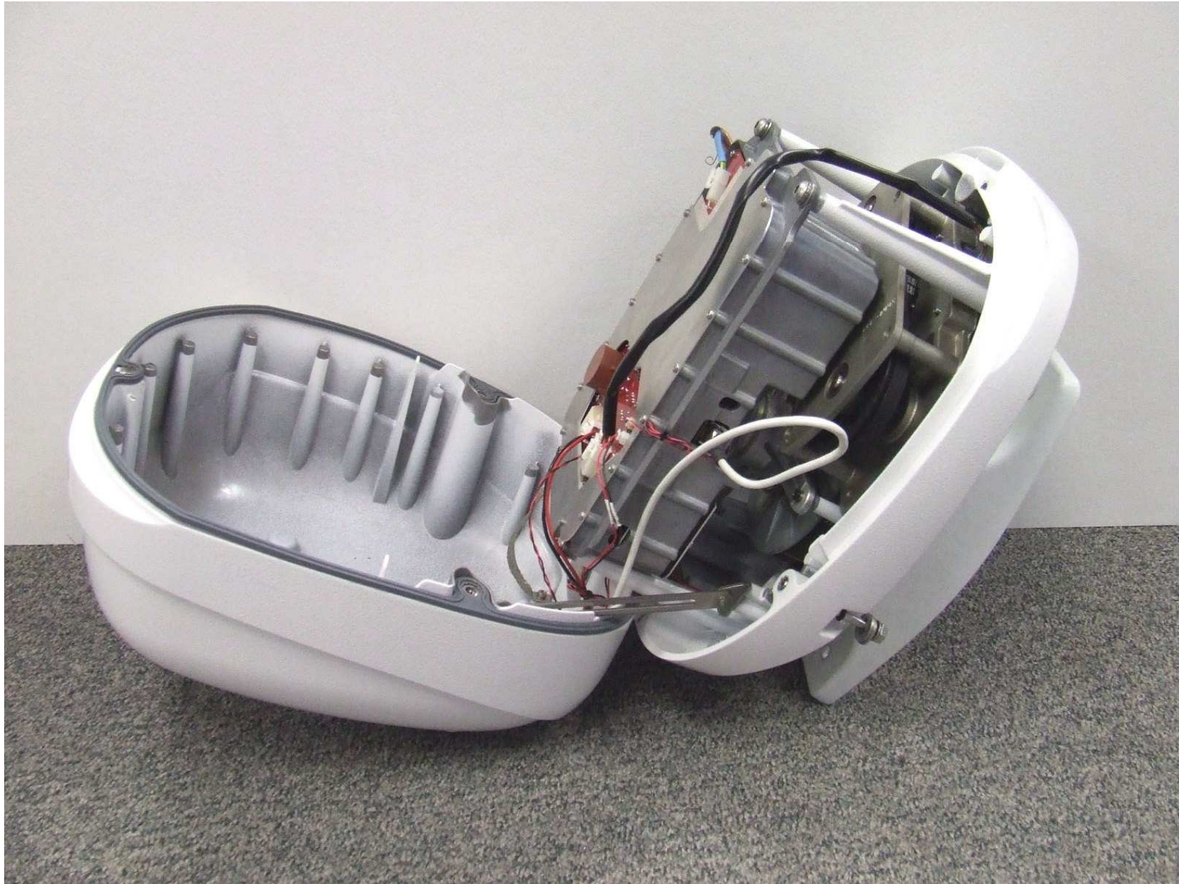
NGS 4kW Digital Open Array Radar Scanner - right-hand view - opened to service position
