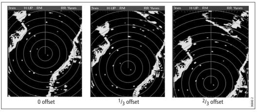
The default mode for the radar application is Relative with zero offset.
