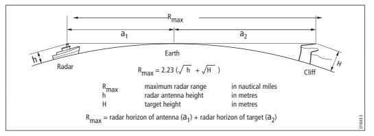
The table below shows typical maximum radar ranges for various radar antenna heights and target heights. Remember that although the radar horizon is greater than the optical horizon, the radar can only detect targets if a large enough target is above the radar horizon.
