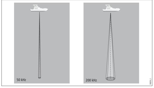
To display the transducer cone:
