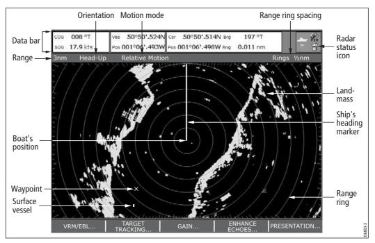
Typically, your boat's position is at the centre of the display, and its dead ahead bearing is indicated by a vertical heading line, known as the Ship's Heading Marker (SHM).
