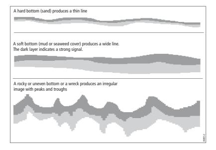
The dark layers indicate a good echo; the lighter areas weaker echoes. This could mean that the upper layer is soft and therefore allowing sound waves to pass to the more solid layer below.
