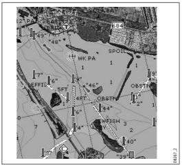
On Land and Sea - displays an aerial photo on both the land and sea areas. This enables you to interpret deeper water (dark blue) from shallower (light blue) and to view land features simultaneously. In shallow water, in some parts of the world where the photos are good and clear you will actually see bottom features like sandbanks, reefs etc.
