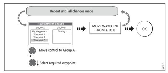
**Note:** Alternatively, waypoints can be moved from Group B to Group A if required. The soft keys reflect this accordingly.
