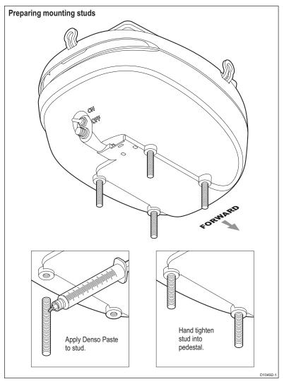
Note: If the studding supplied is not long enough for the mounting surface thickness, use M10 stainless steel, grade A4-70 studding of a suitable length. Refer to the following illustrations for details.
