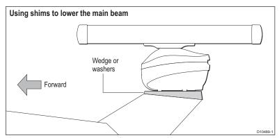
The shims may be made from aluminium plate wedges, simple flat washers, or an angled wooden block. For thick shims, you may need longer securing bolts than the M10 studding supplied, (see note in Installing the Digital Radar Components on p.26).
