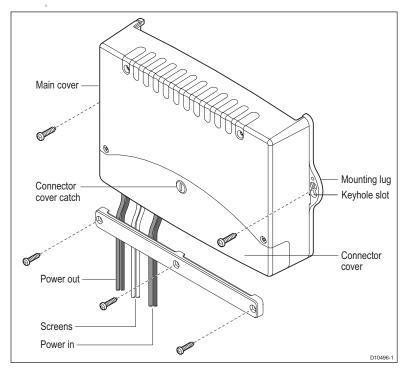
Ensure the VCM100 unit is level on it's horizontal plane. Once situated, fit in position with the 2 mounting screws provided
