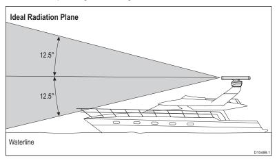
Planing hull vessels, and some displacement hull vessels, adopt a higher bow angle when the vessels is at its cruising speed. In many cases this substantially alters and raises the radar's main radiation plane, and can cause poor detection of nearby targets. It may be helpful to lower the radar beam back towards the parallel, by shimming the rear of the digital radar, so that the beam points slightly downwards with respect to the waterline when the vessel is at rest.
