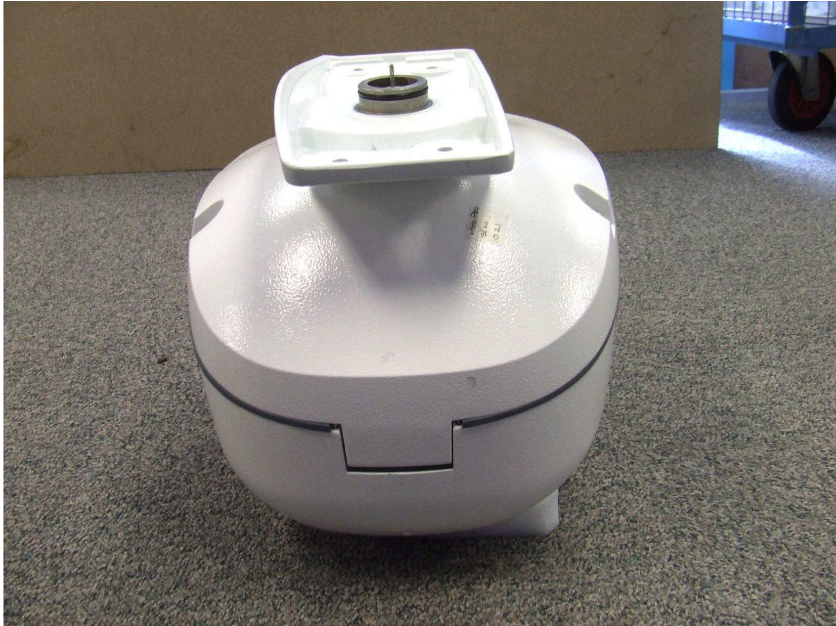
NGS 4kW Digital Open Array Radar Scanner - front view
