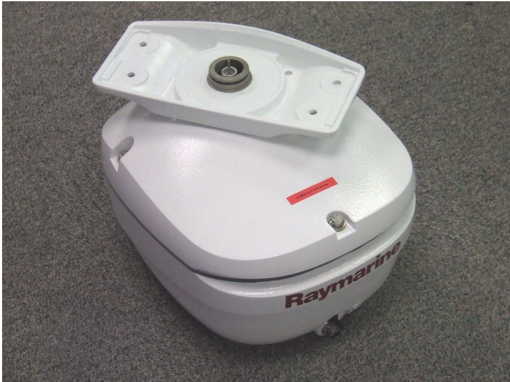
NGS 4kW Digital Open Array Radar Scanner with Antenna and power/ethernet cable removed
