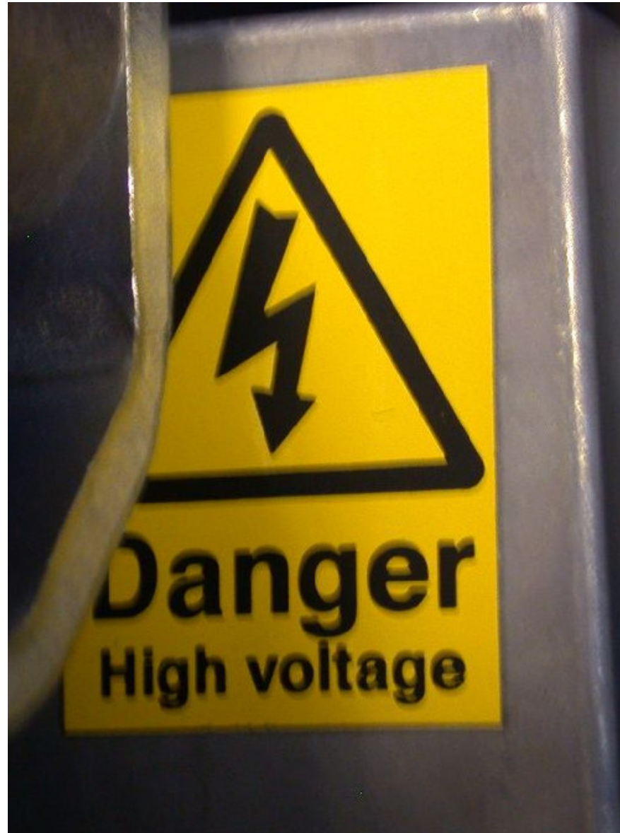
Warning label used on the core casting near the magnetron (3029-193-A)
