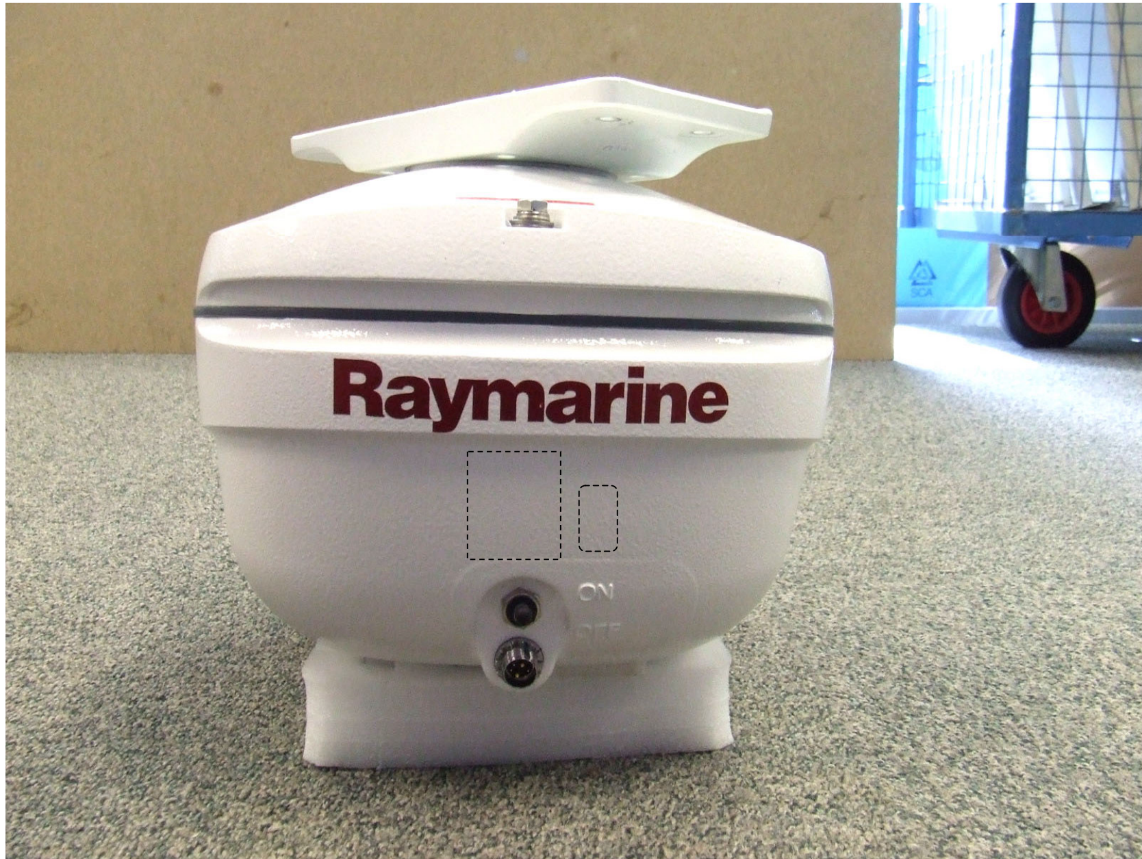
Expanded view showing intended position of approval and ratings labels Page 5 of 9
