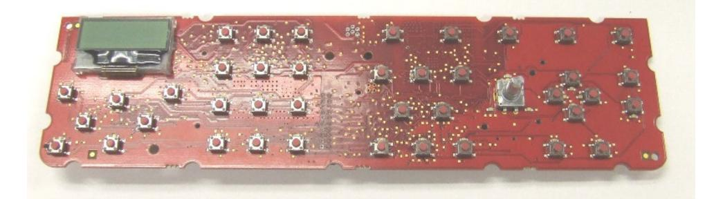
INTERNAL VIEW PCB, keyboard switch side
