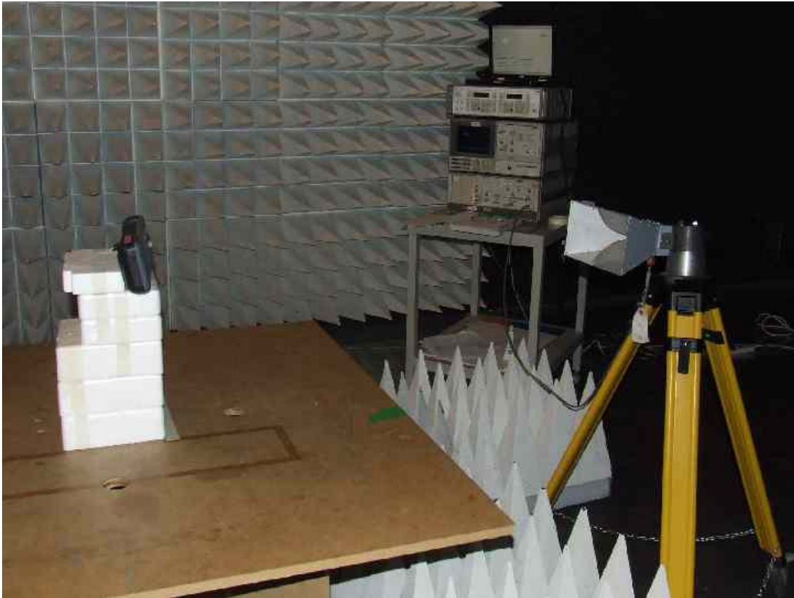
Figure 3 Set up showing measurements above 7GHz at 1m. Antenna shown is for measurements up to 18GHz.
