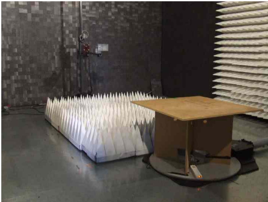
Figure 1 View from within chamber showing turntable, base and mast set-up for measurements from 1 - 40GHz. Antenna shown covers 1 - 18GHz. Floor absorber is removed for tests below 1GHz.
