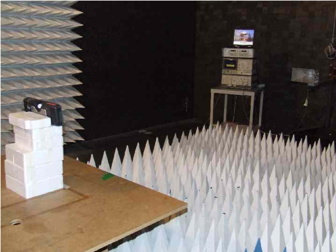
Figure 2 Set up in chamber for 2 – 7GHz measurements at 3m.
