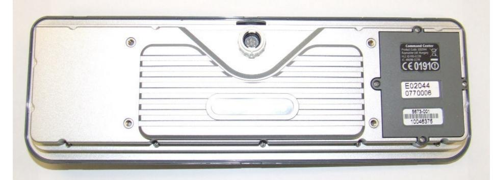
Rear view showing STNG connector (for battery charging or wired use) and with rear installation clamp/outer cover removed
