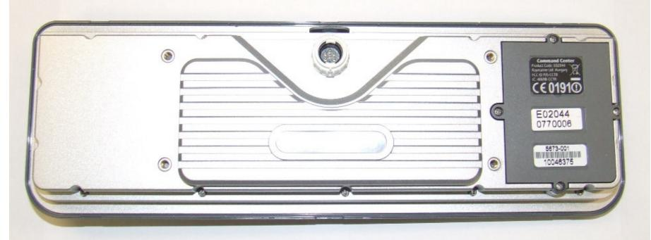
Rear view of keyboard showing position of labels on battery compartment cover
