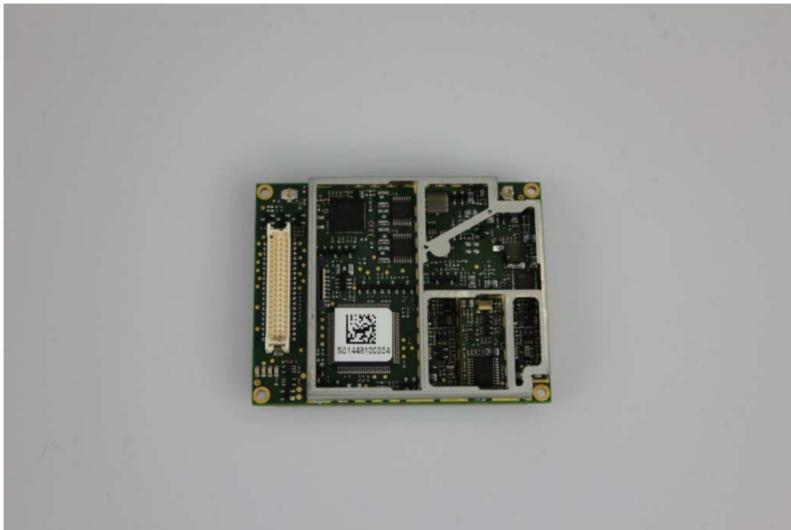
Figure 5 – TLA Module, Top View with no EMC CAN
