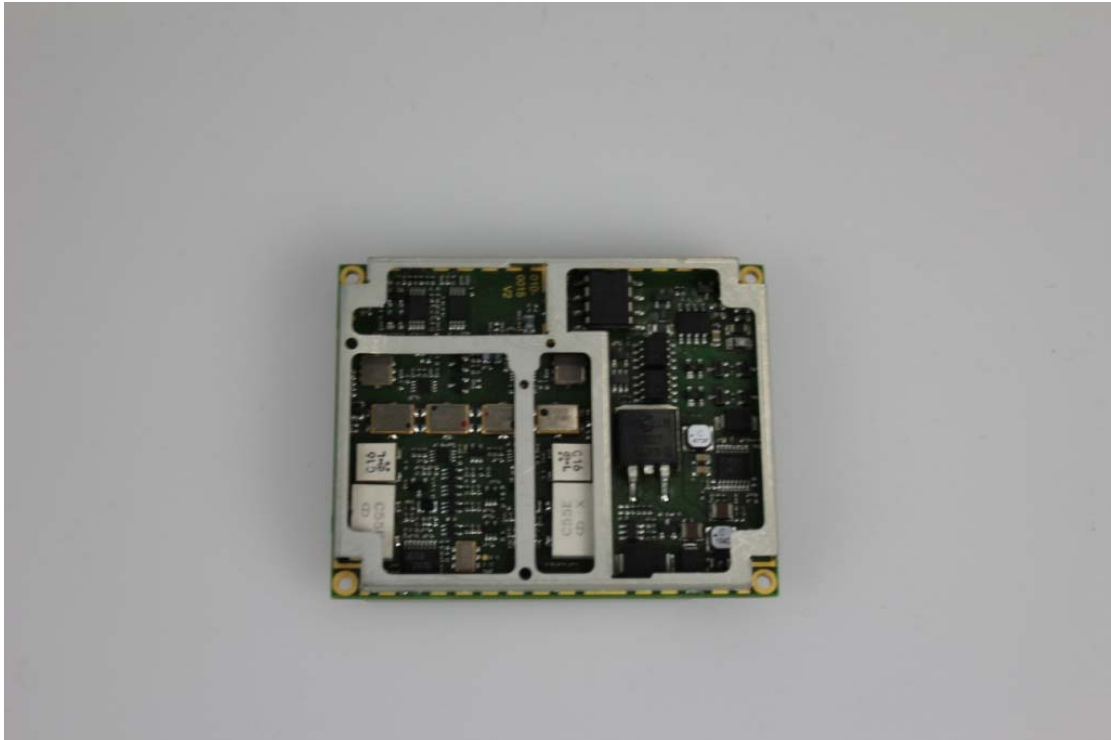
Figure 6 – TLA Module, Bottom View with no EMC CAN
