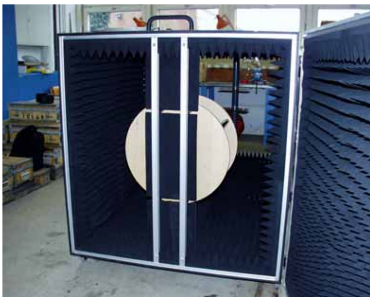
GPS test box, interior view
