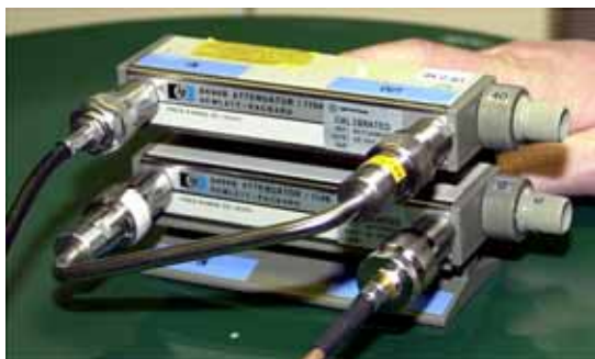
Calibrated attenuation cell, connector side
