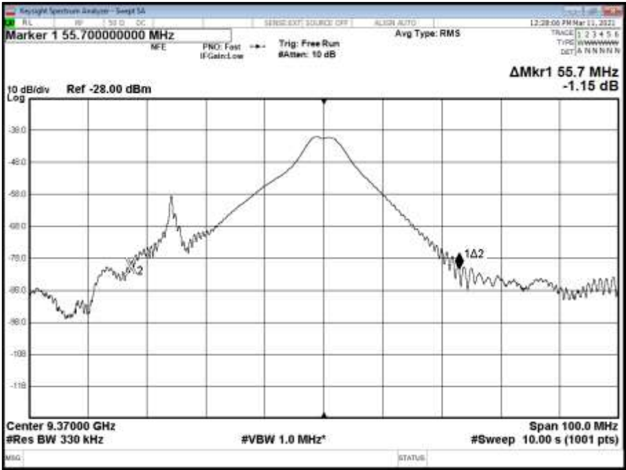
Figure 48 - 9370, FM, 750 ns, 40 dB Bandwidth
