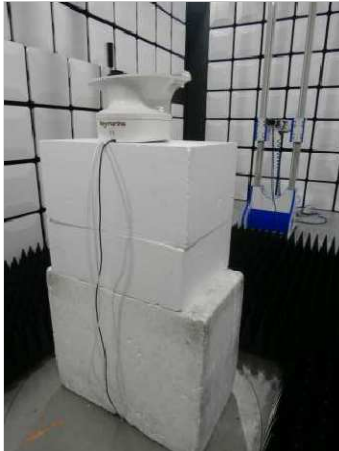
Figure 76 - Test Setup - 1 GHz to 18 GHz
