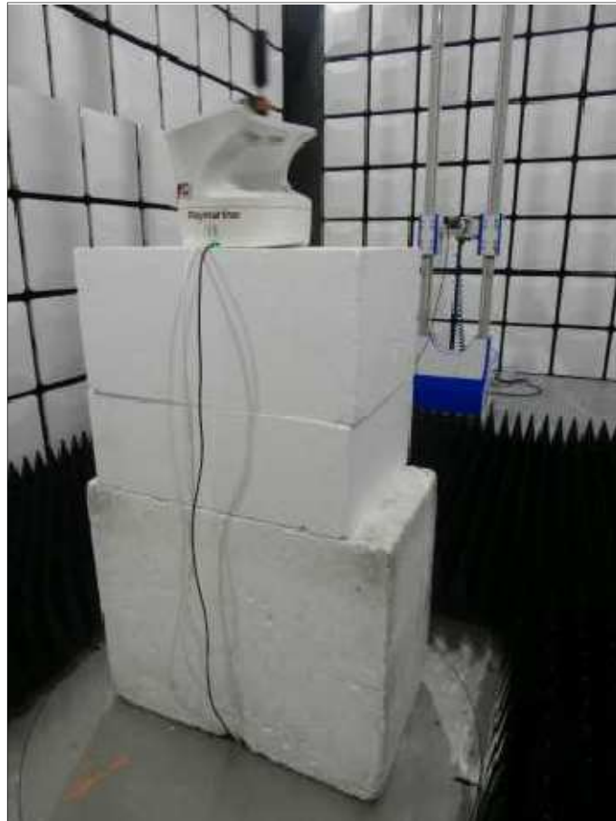
Figure 77 - Test Setup - 18 GHz to 40 GHz
