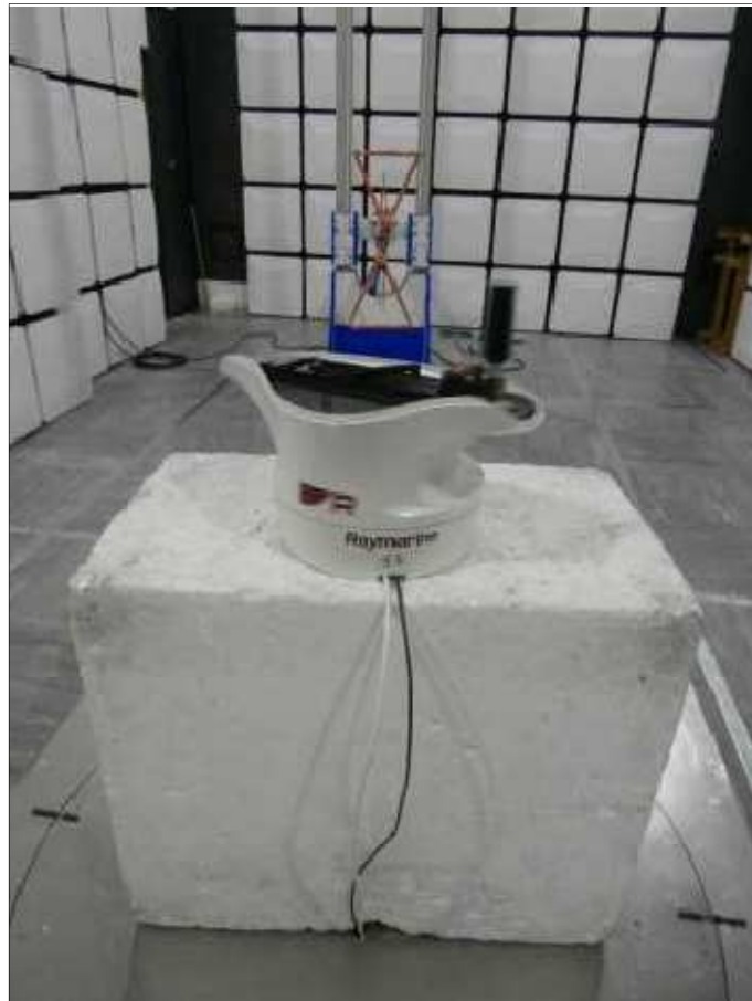
Figure 75 - Test Setup - 30 MHz to 1 GHz
