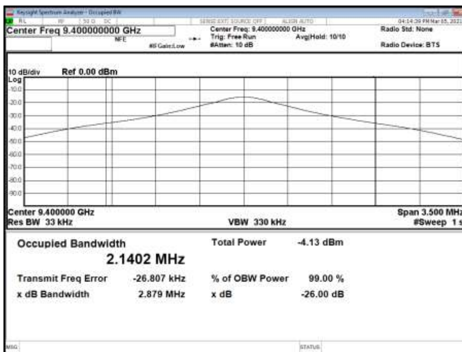
Figure 41 - 9400 MHz, FM, 35000 ns, 99% Occupied Bandwidth
