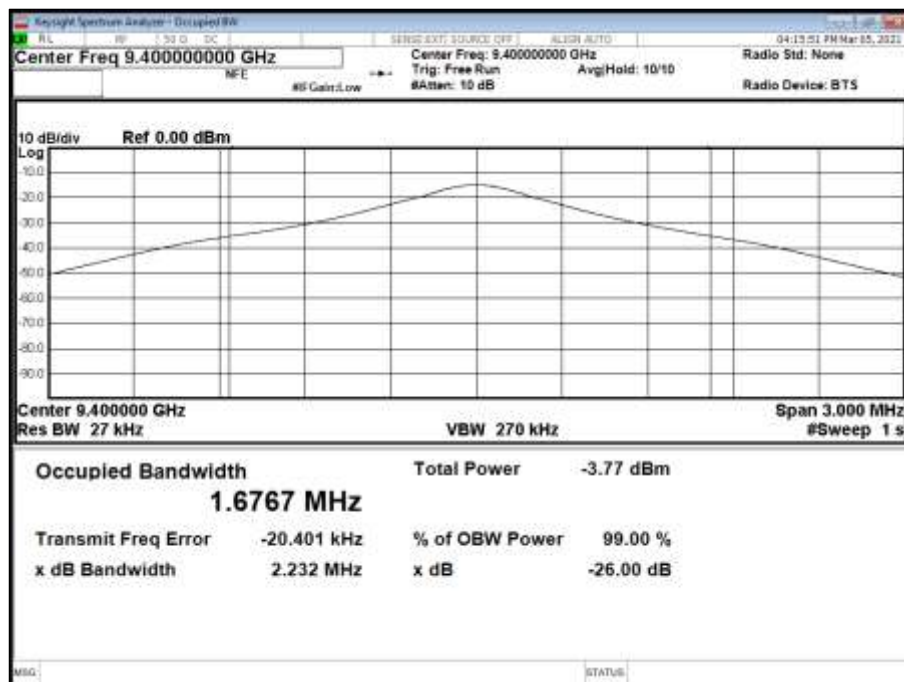
Figure 43 - 9400 MHz, FM, 47000 ns, 99% Occupied Bandwidth
