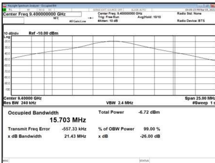
Figure 33 - 9400 MHz, FM, 2710 ns, 99% Occupied Bandwidth
