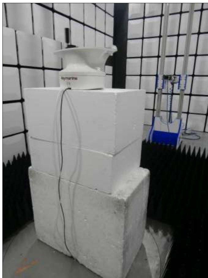
Figure 76 - Test Setup - 1 GHz to 18 GHz
