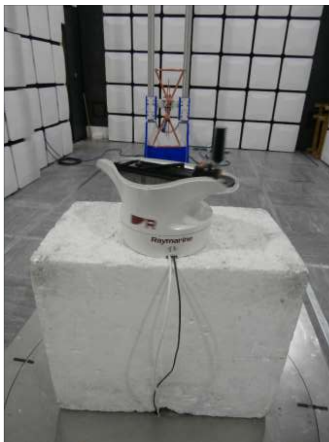
Figure 75 - Test Setup - 30 MHz to 1 GHz
