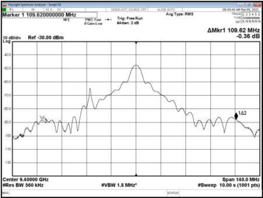
Figure 22 - 9400 MHz, FM, 192 ns, 40 dB Bandwidth
