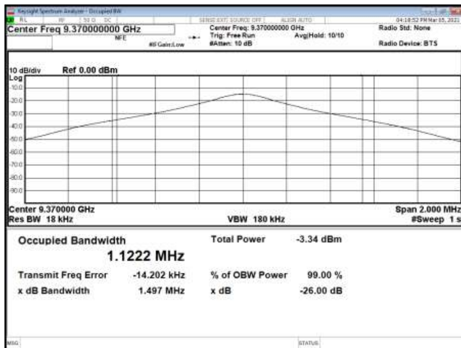
Figure 49 - 9370, FM, 79000 ns, 99% Occupied Bandwidth
