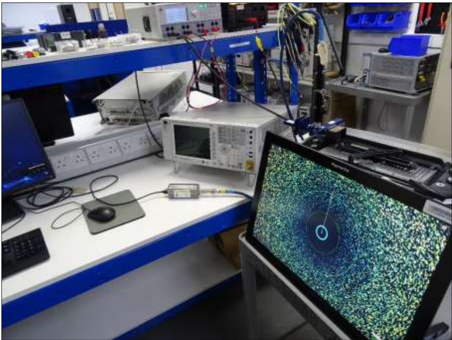
Figure 78 - Conducted Test Setup
