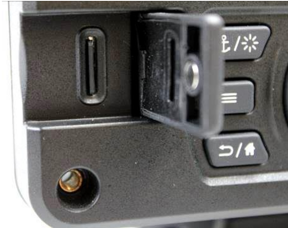
Figure 5 – SD Card location
