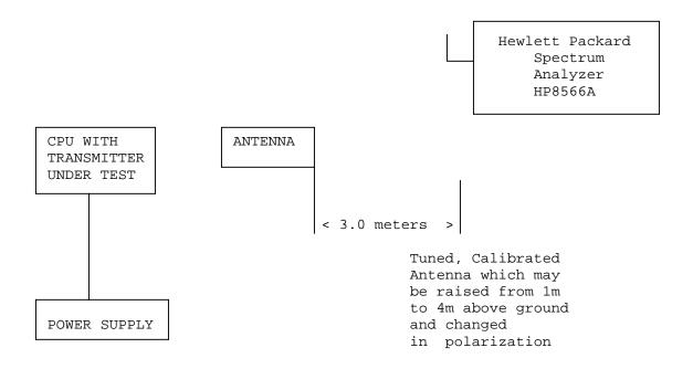
Equipment placed 80 cm above ground on a rotatable platform.
