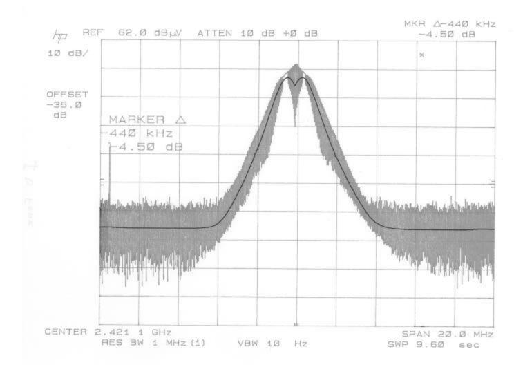
The correction for peak to average radiated is 4.50 dB. The above plot shows the peak to average signal displayed.
