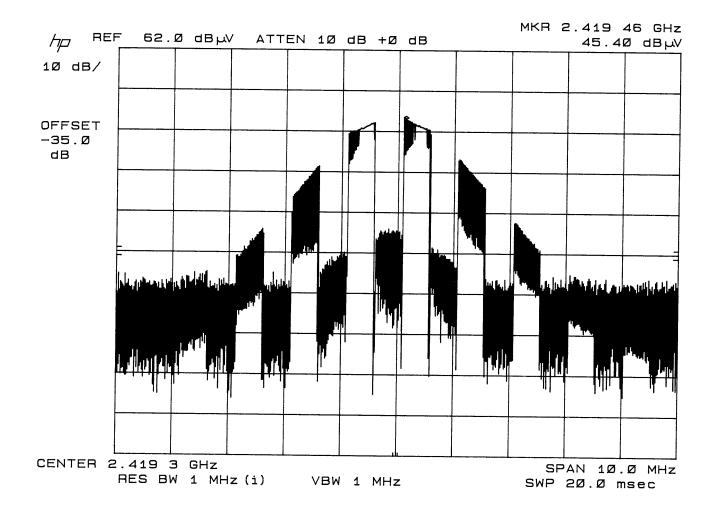
The duty cycle correction factor was calculated from the above modulation envelope. The pulsed output wave form calculation shows a 50% duty cycle for a 6.02 dB correction factor.
