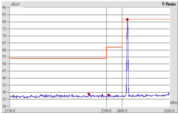
This is the hard copy of our bandedge measurement generated by our bandedge testing program. The plot shown above is the bandedge of channel 1 of base.
