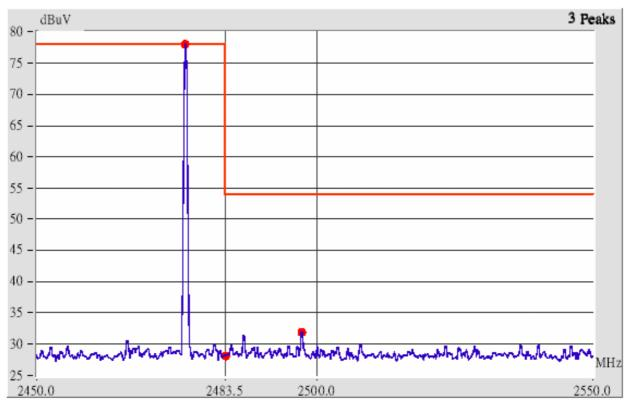
This is the hard copy of our bandedge measurement generated by our bandedge testing program. The plot shown above is the bandedge of channel 40 of handset.
