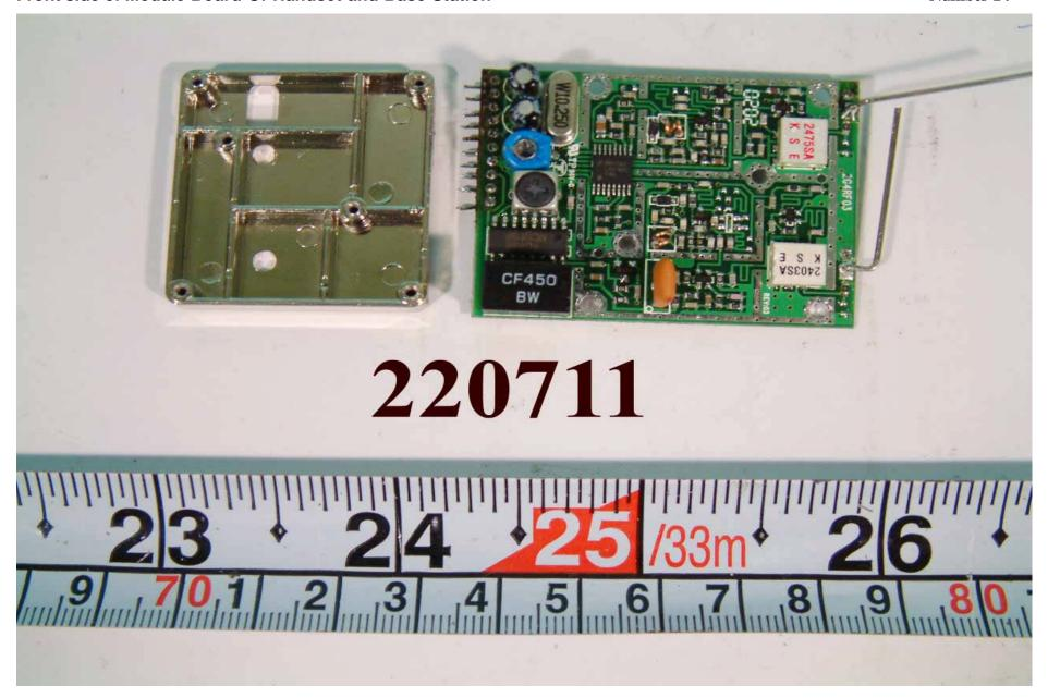
Front side of Module Board Of Handset and Base Station
