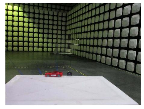
1.1 Radiated Emissions (30MHz-1GHz) Test Setup
