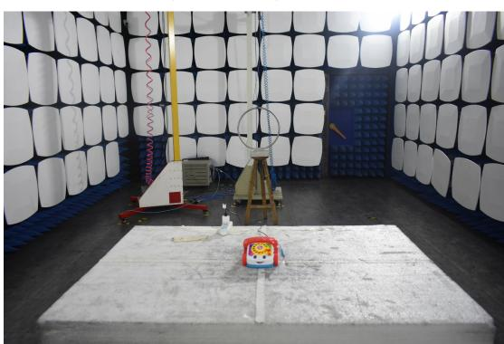
3. Radiated emission (9KHz-30MHz)
