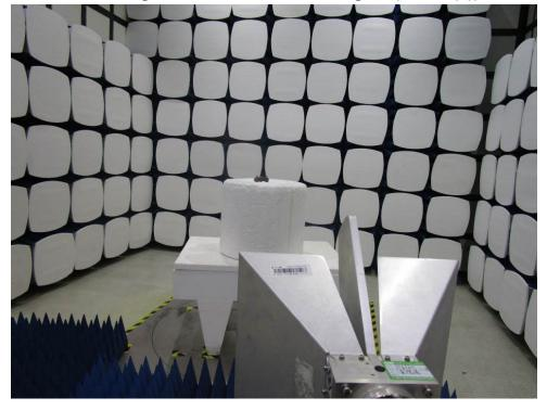
1.1 Field Strength of the Fundamental Signal (15.249(a)) Test Setup
