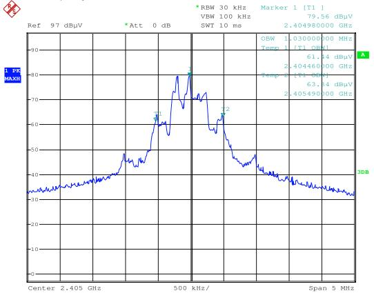
According to above plot, 20dB bandwidth falls in assigned band (2400-2483.5)MHz. It is deemed to comply with section 15.215
