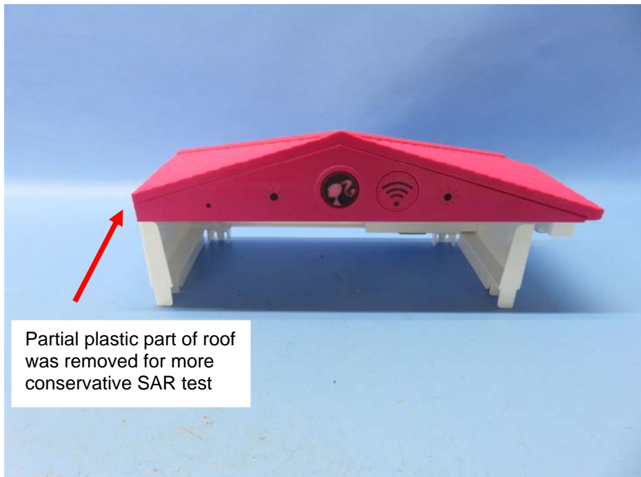
Figure 4 – Modified Front view (Roof Unit)
